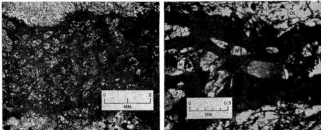
FIG. 3. Photomicrograph displaying the full width of one of the dark veins in Catherwood.
